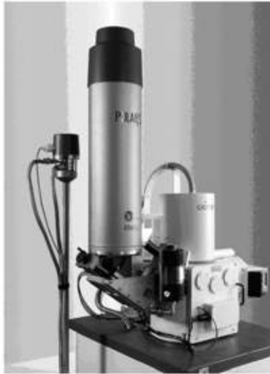
Fig. 3. Polar microcalorimeter energy dispersive X-ray spectrometer.
